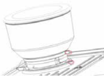
Fig. 2: Align the positions in red circles in the Figure, and press it down, rotate it clockwise and install it into the machine.
